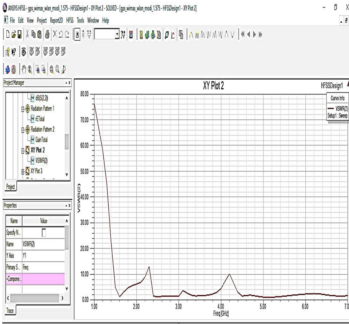
**Figure 4.3** Simulation output of VSWR
