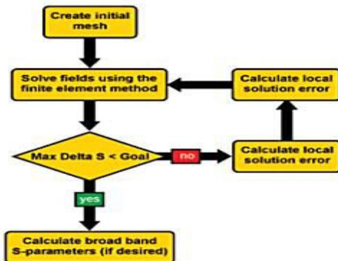
Figure 3.2 Flow Diagram of Simulation Process
