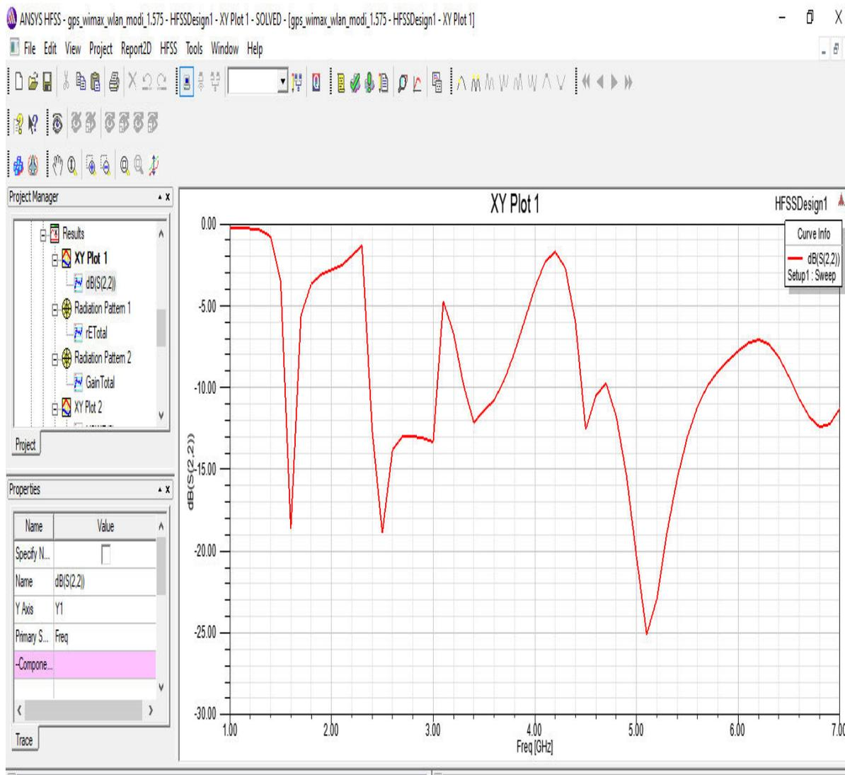
**Figure 4.6** Simulation Output of Return Loss
