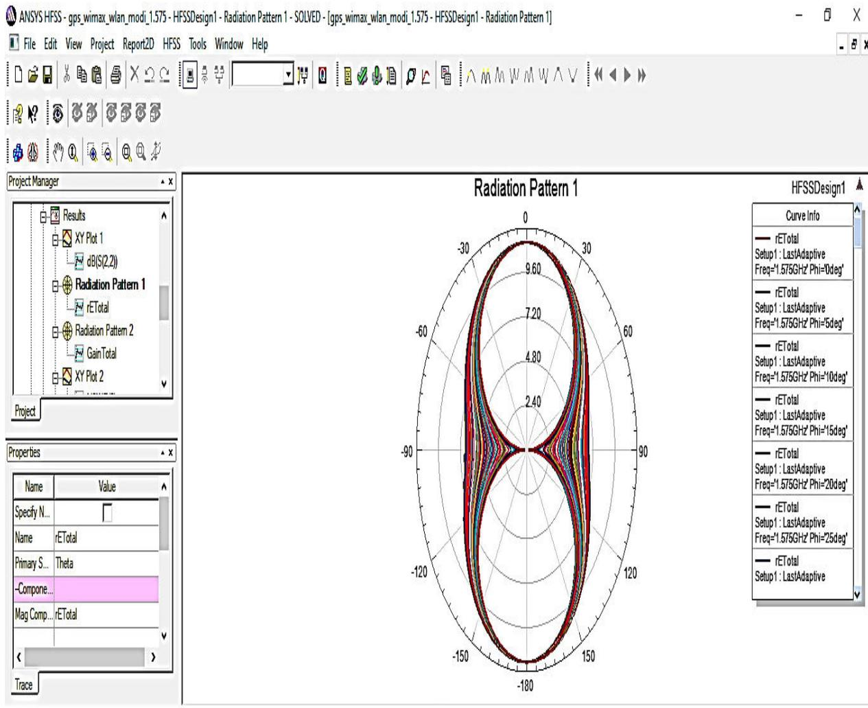
Figure 4.5 Simulation Output of Radiation Pattern
