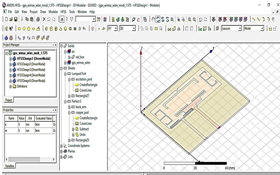
Figure 4.2 Top View of Rectangular Antenna Design
